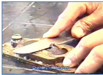
Figure 14.3 Molding and Cutting of Test Specimen
