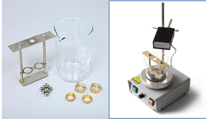
Figure 12.1 Ring and Ball apparatus
