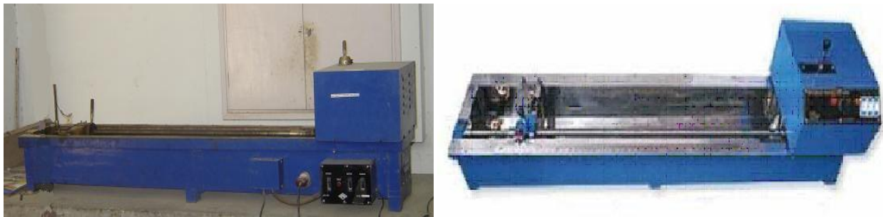
Figure 14.2 Ductility Testing Machine
