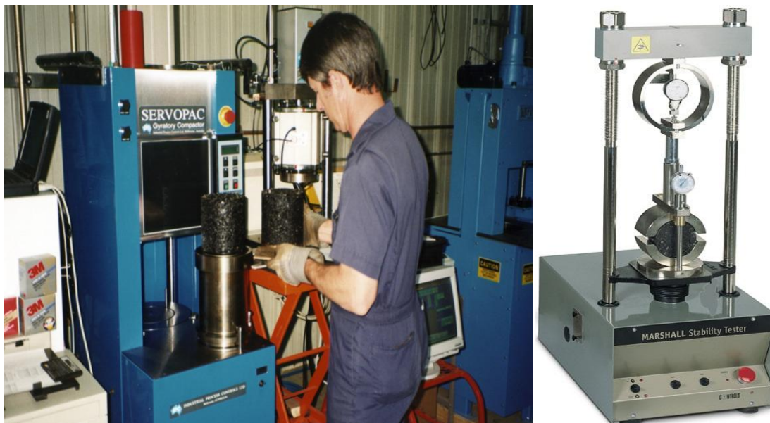
Figure 17.5 Marshall stability and flow test
