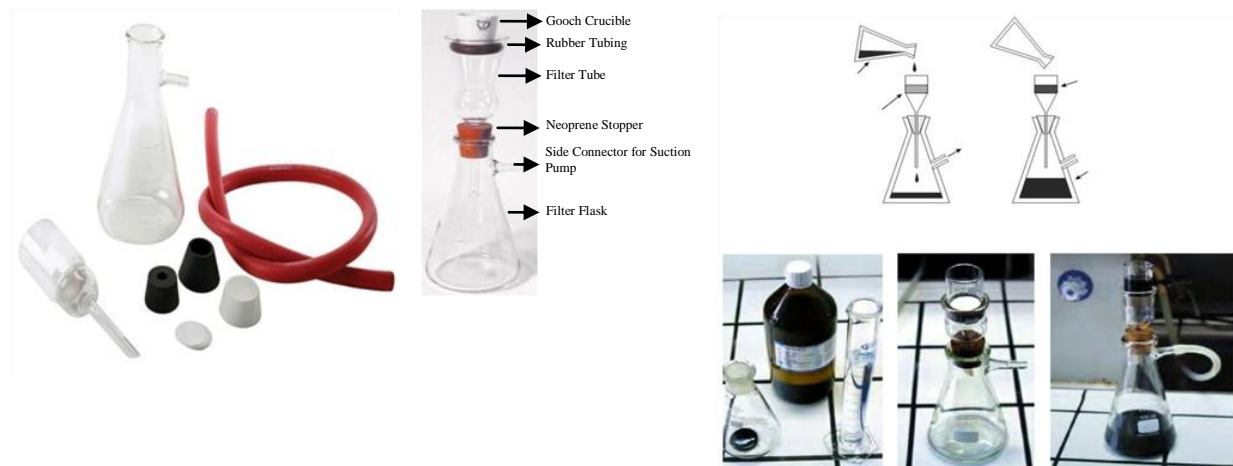
Figure 13.1 Component parts of the filtering apparatus
